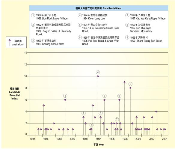
圖41. 1984年至今引致山泥傾瀉警報的暴雨。 Figure 41. Chart showing rainstorms since 1984 that resulted in the issue of landslip warning.
