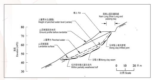
圖B-6. 用作斜坡穩定性分析的事發地點代表性剖面圖 - 上部匙形滑動。 Figure B-6. Representative cross-section of the landslide for slope stability analyses - upper spoon-shaped slip.
