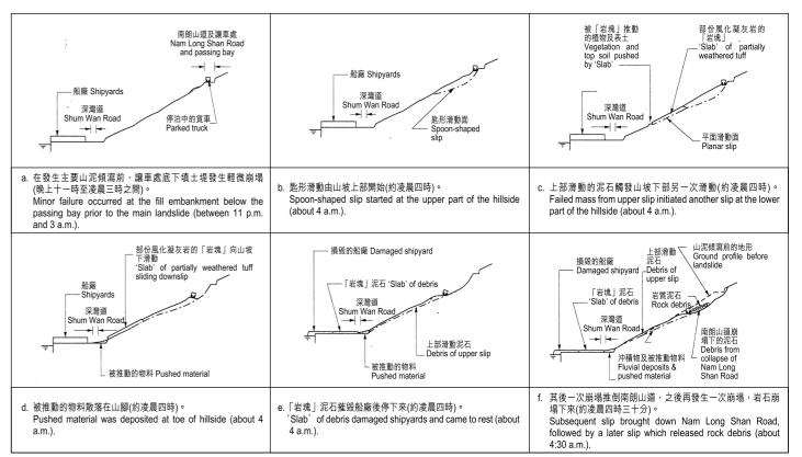
圖B-10. 山泥傾瀉過程的圖解説明。 Figure B-10. Schematic representation of inferred sequence of events.
